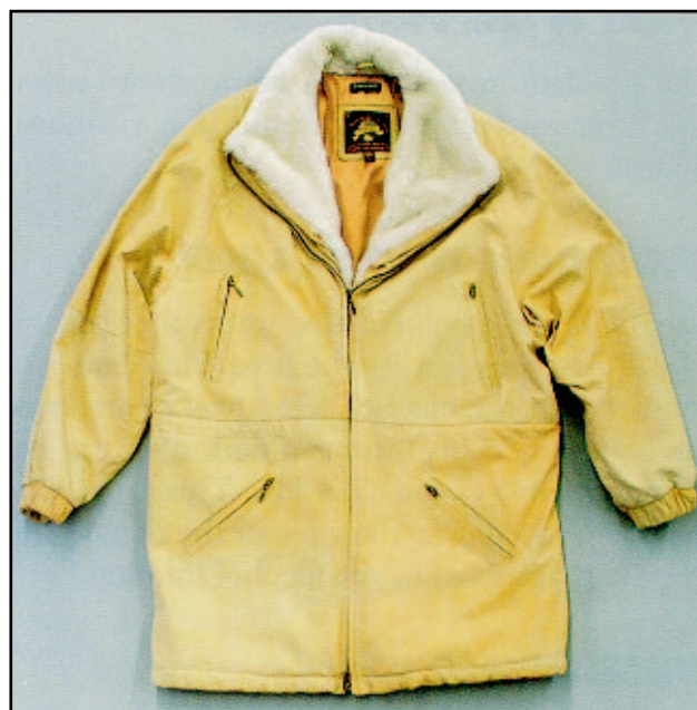
The left panel of this leather jacket is noticeably lighter than the right panel. Severe color losses on leather or suede are due to poor manufacturer selection of dyes, oils, and finishes.
