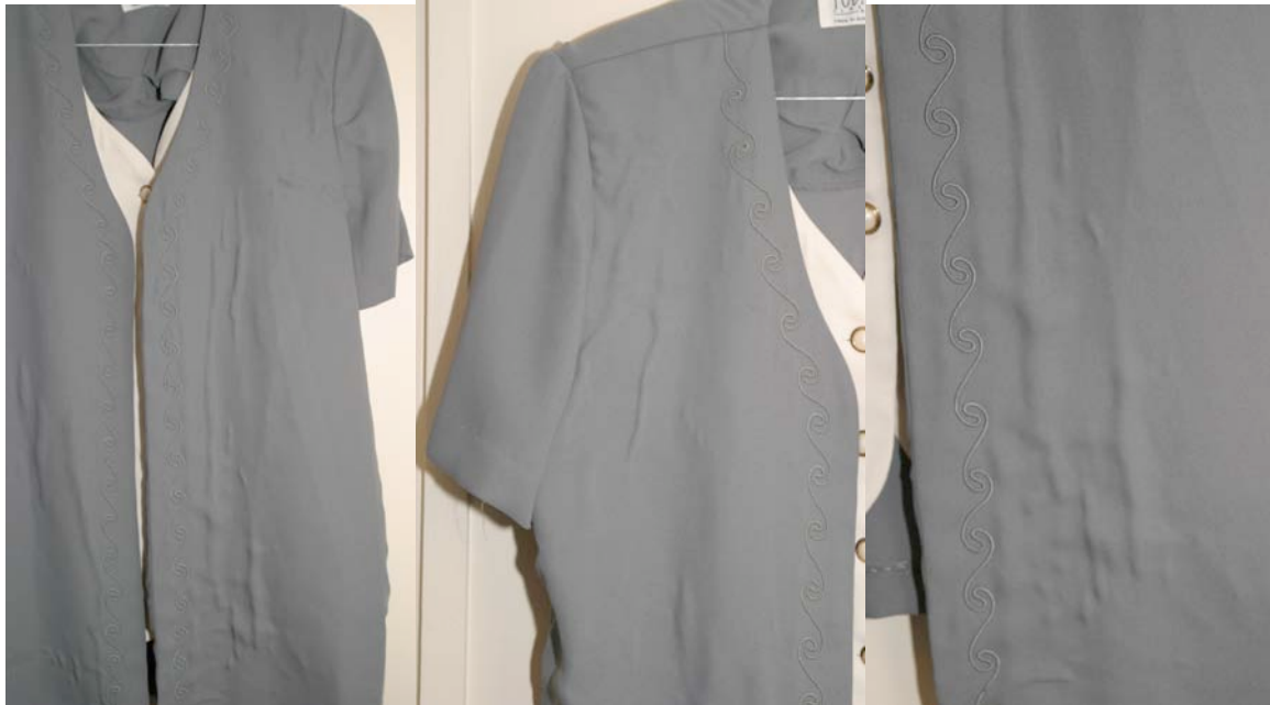
Various Views Of The Front Of The Garment Showing The Blistering Or Bubbling Effect Caused By The Failure Of The Fusible Interlining
