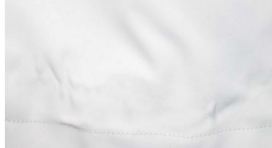
Photograph 3. Blistering Above the Hem Area
